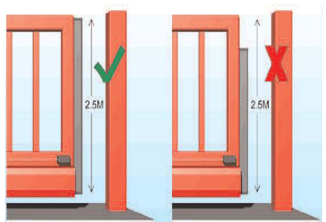
Figure 2 – safeguarding required up to 2.5m from ground level
